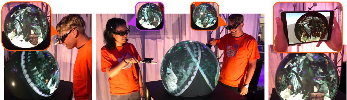
Figure 1: Our multi-person spherical FTVR display. From left to right (users' views inset): a single person viewing a fishbowl scene with perspective-correction and stereo, two people collaborating with two independent perspective-corrected views of the same scene, and a third person using a tracked mobile screen to get a perspective-corrected augmented reality view.
